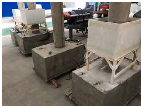
Fig. 3. Actual corrosion of the test specimens.
